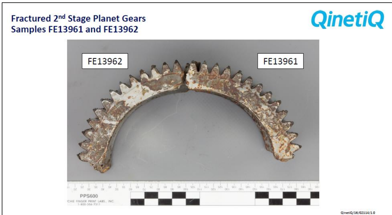
Figure 2: The two pieces of the second stage planet gear prepared for metallurgical examinations. Photo: QinetiQ
